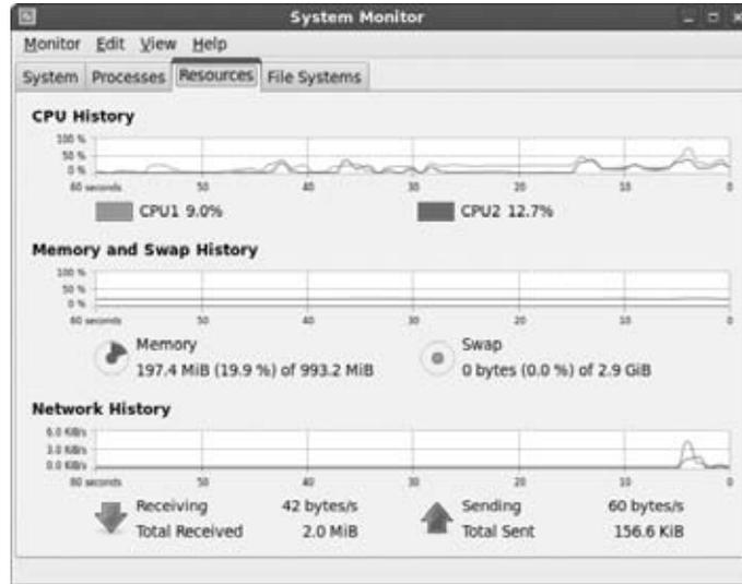
**Figure 8-3:** The System Monitor displaying CPU, memory, swap, and network usage
