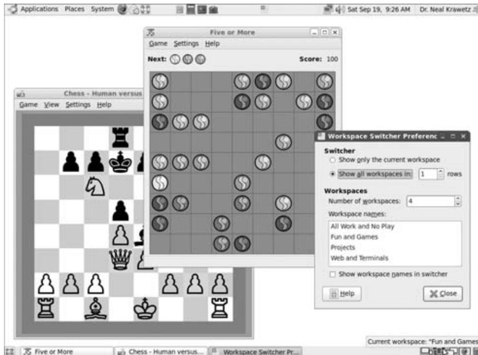
**Figure 9-3:** The Workplace Switcher in the lower-right corner, showing four distinct desktops
