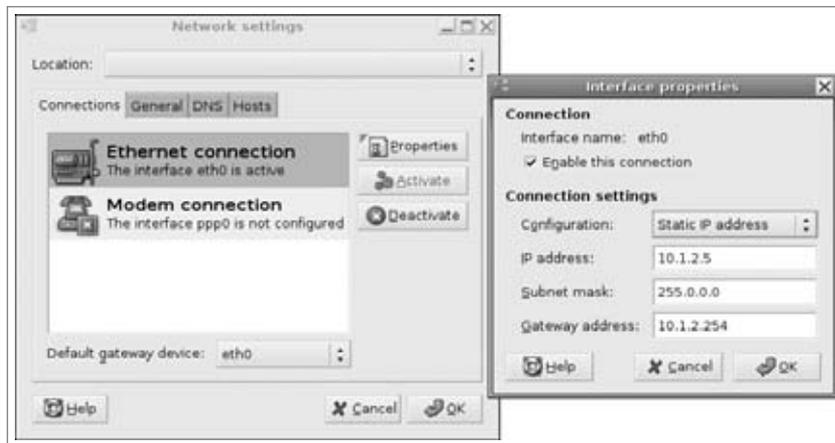
**Figure 12-1:** The Network Settings applet under Dapper Drake, showing the properties for eth0
