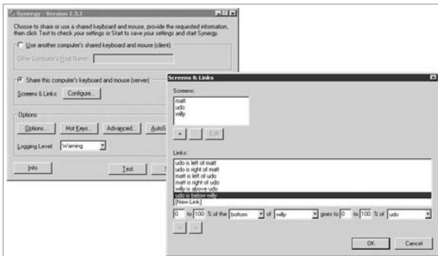
**Figure 10-10:** The Microsoft Windows Synergy server configuration window showing the same relationships as Listing 10-3
