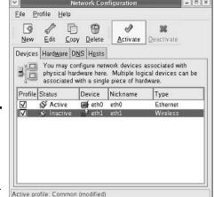
Figure 3-7: Activate the new wireless device from this window.
