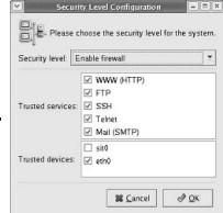
Figure 3-5: You can set up packet filtering with this tool.
