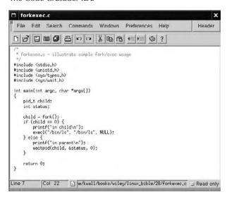
As you can see in Figure 28-4, Code Crusader has a much simpler, cleaner interface than the other IDEs mentioned so far. Another significant difference between Code Crusader and the larger IDEs such as Eclipse and KDevelop is that each IDE component, such as the project browser, the class browser, editor windows, and the log viewer, opens in its own, independent window rather than being part of a single-document interface (SDI).
