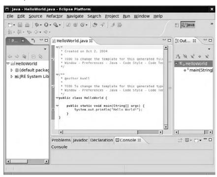
Figure 28-1 illustrates a number of characteristics typical of IDEs. The project view on the left side of the screen provides a project file browser that enables you to see at a glance the contents of the programming project. You can see the primary project folder, HelloWorld, and some of the associated files necessary to support Java projects, such as the default package for Java projects and a folder containing the necessary JRE (Java Runtime Environment) files.
