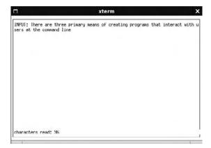
Ncurses-based programs can also read input piped from stdin. Figure 28-6 shows the results of the command cat /etc/passwd | ./nreadkey.
