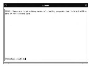
As you can see from Figure 28-7, the basic appearance and functionality of sreadkey.c is the same as nreadkey.c. The differences between the two, which have to do with the TUI framework used to create sreadkey.c, are invisible to the user. S-Lang—based programs can also read input piped from stdin.
