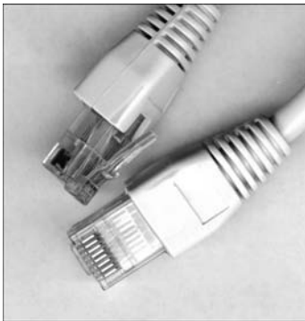
Figure 15-8: A star topology's twisted-pair cables have RJ-45 connectors (similar to telephone-cable connectors).
