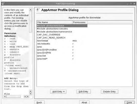
Figure 2.43 AppArmor Profile for Netstat
