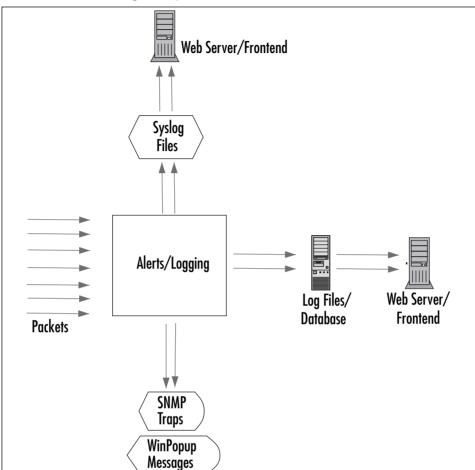
Figure 4.5 Snort's Alerting Component.
