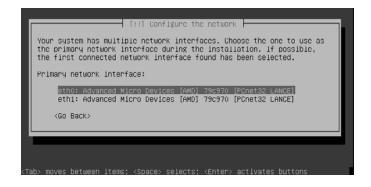
Figure 5-10 Selecting the primary network interface
