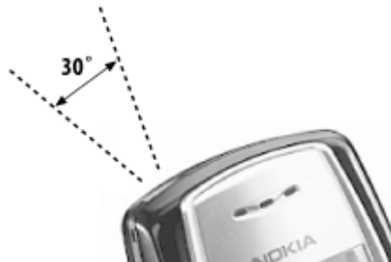
Figure 8-1. The 30-degree cone for peak power intensity of an infrared port
