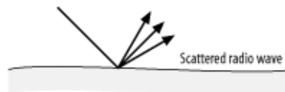
Figure 1-4. Scattering of a radio wave
