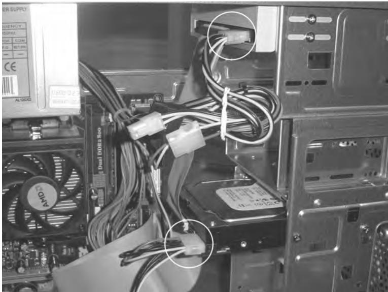
**Figure 1-27.** The Molex cables are connected to the CD/DVD drive and hard drive.
