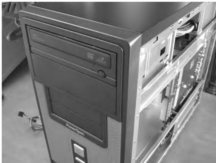
**Figure 1-17.** Insert the CD/DVD drive into the open bay slot.
