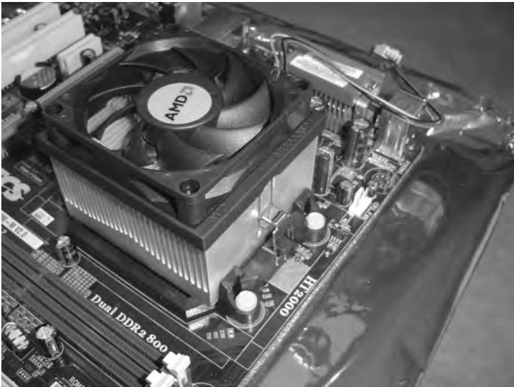
**Figure 1-5.** *Install the processor's cooling fan as described in the processor's documentation.*
