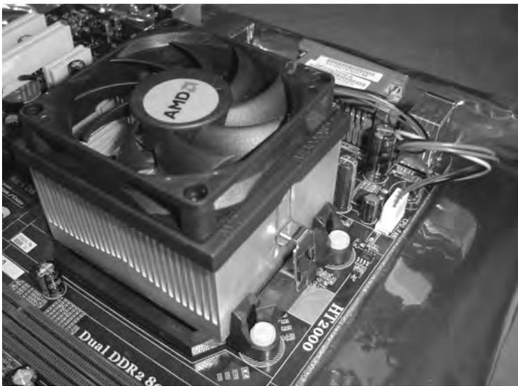
**Figure 1-6.** *The cooling fan gets its power from the motherboard.*
