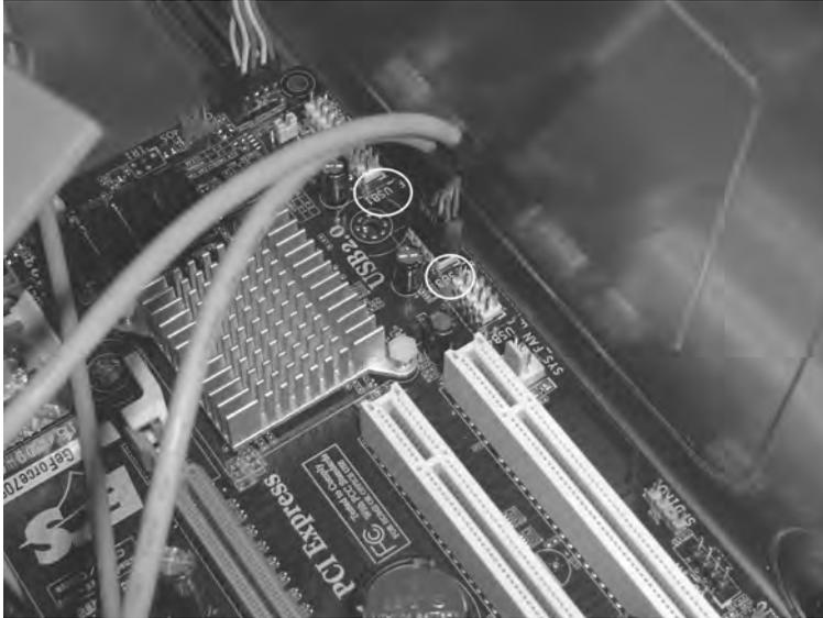
**Figure 1-30.** Plug in the USB cable to one of the USB connectors.
