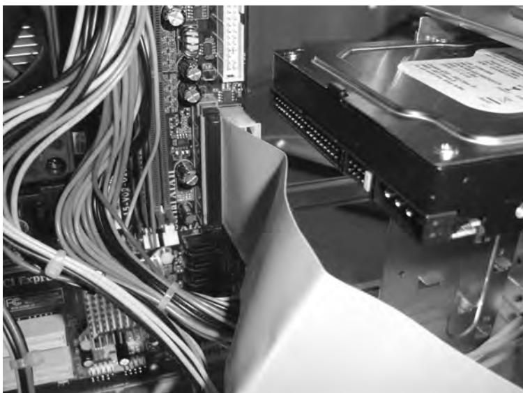
**Figure 1-24.** *Connect the CD/DVD and hard drive cable to the motherboard.*
