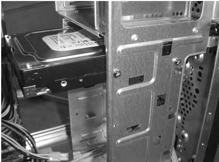
**Figure 1-19.** Use screws to securely connect the hard drive to the case.
