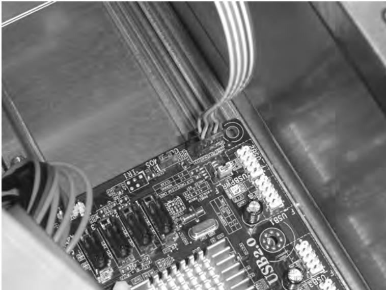
**Figure 1-29.** *Plug in the case's power button and light controlling cable.*
