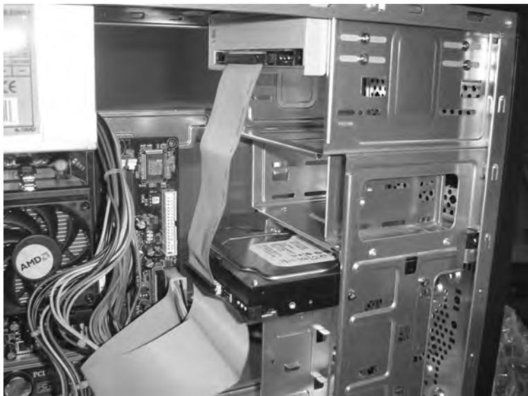
**Figure 1-25.** *The data cable is connected to the CD/DVD drive and hard drive.*
