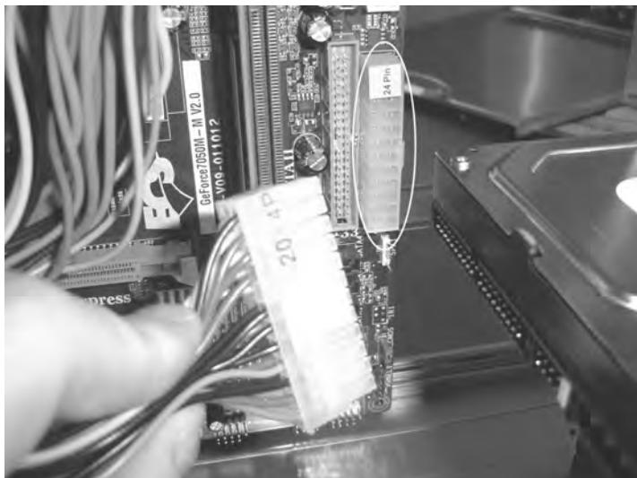
**Figure 1-21.** *The ATX motherboard power connector plugs in here.*
