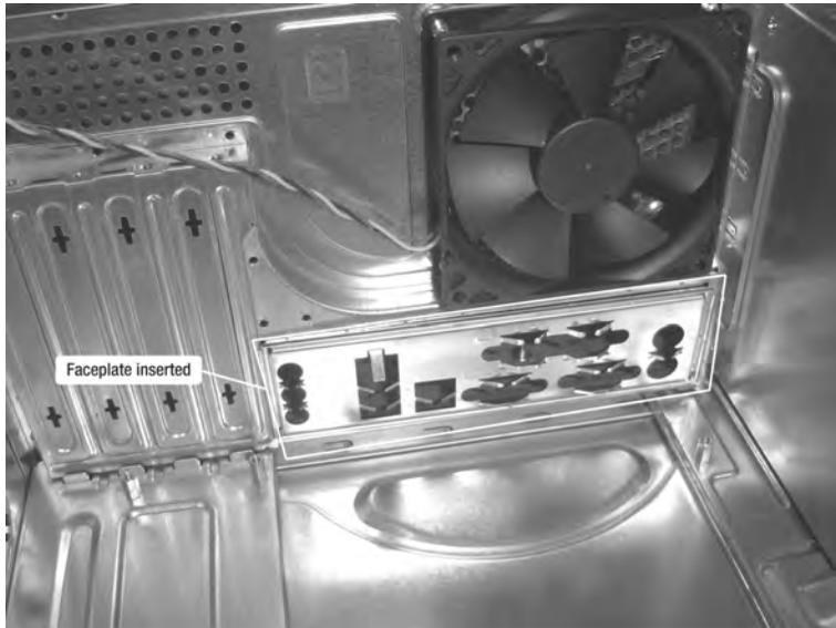
**Figure 1-13.** *The faceplate must be inserted in the case before connecting the motherboard.*
