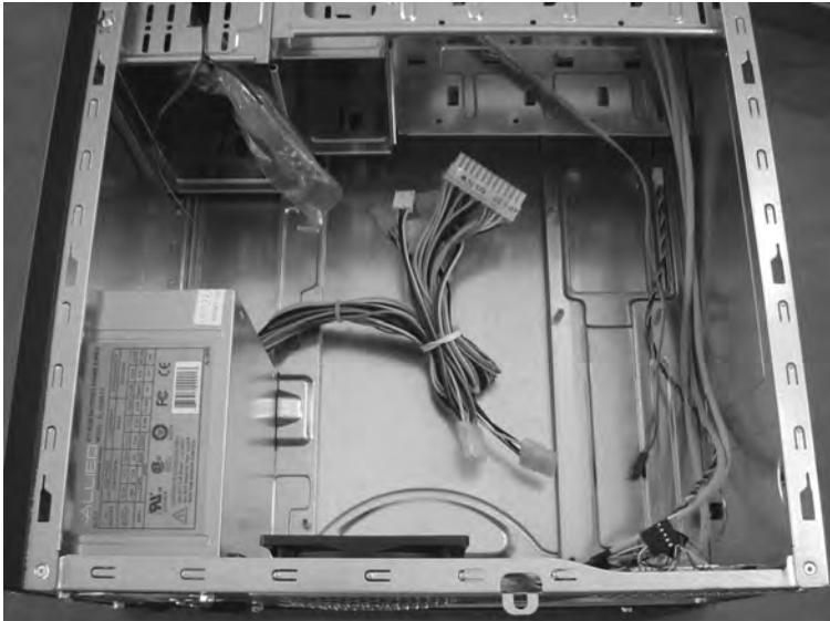
**Figure 1-11.** *The computer case is open and ready for parts to be added.*
