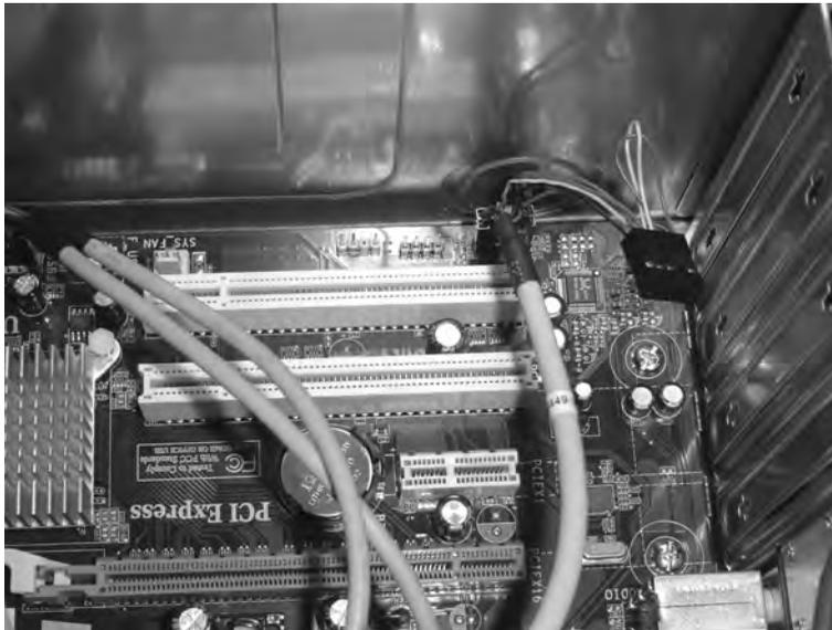
**Figure 1-32.** *Connect the speaker cable to the motherboard.*
