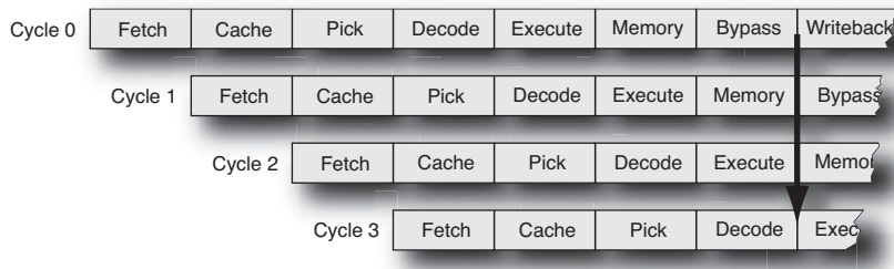
Figure 1.10 Pipelined instruction execution including bypassing of results
