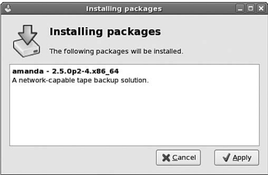
FIGURE 5.1 Installing an RPM Package with Software Installer
