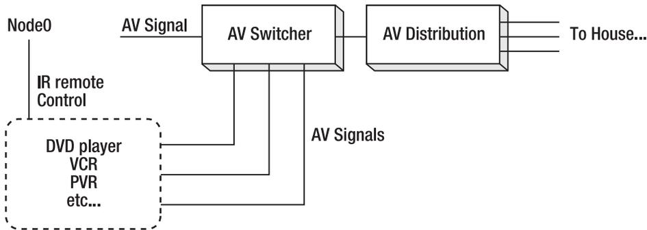
**Figure 7-11.** *Placing all the AV in Node0*
