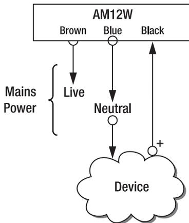
**Figure 2-8.** Connecting an AM12W to a mains-powered device
