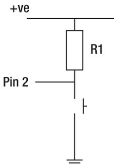
**Figure 2-2.** Reading a digital switch on the Arduino
