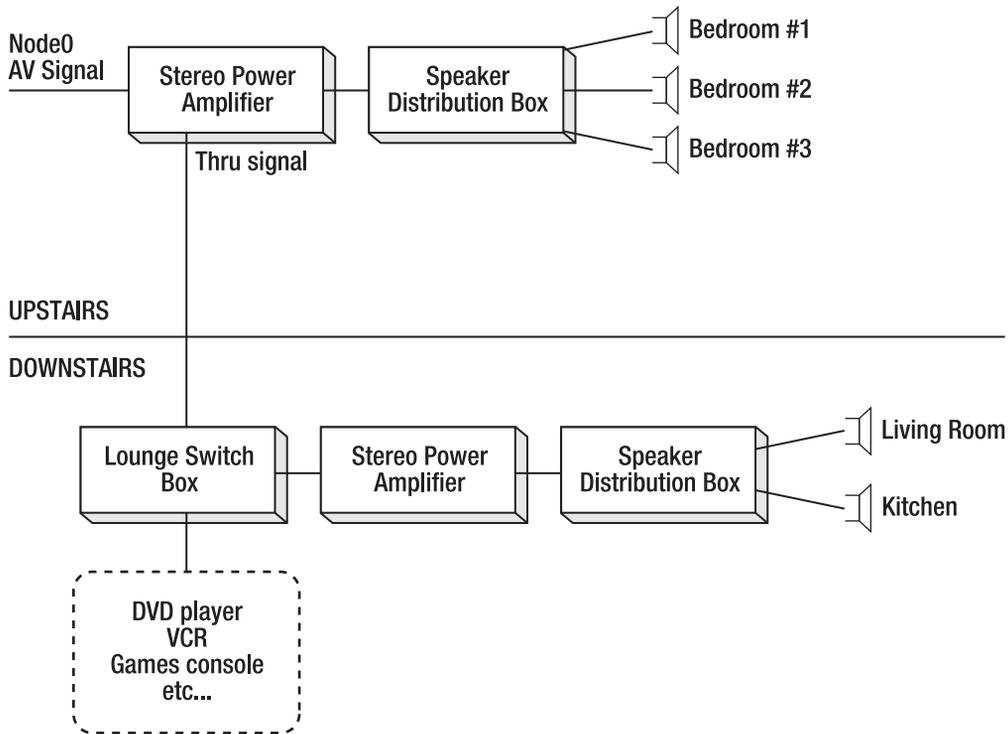
**Figure 7-10.** A simple AV distribution network
