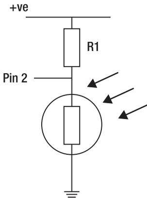
**Figure 2-3.** Reading the light on the Arduino
