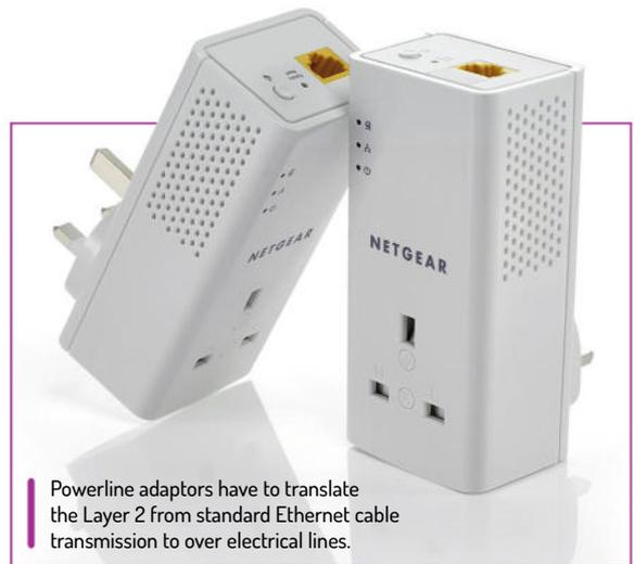
Powerline adaptors have to translate the Layer 2 from standard Ethernet cable transmission to over electrical lines.
