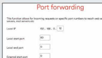
A typical router port forwarding configuration page. The exact procedure varies between manufacturers.
