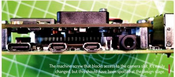
The machine screw that blocks access to the camera slot. It's easily changed, but this should have been spotted at the design stage.
