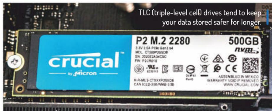
TLC (triple-level cell) drives tend to keep your data stored safer for longer.
