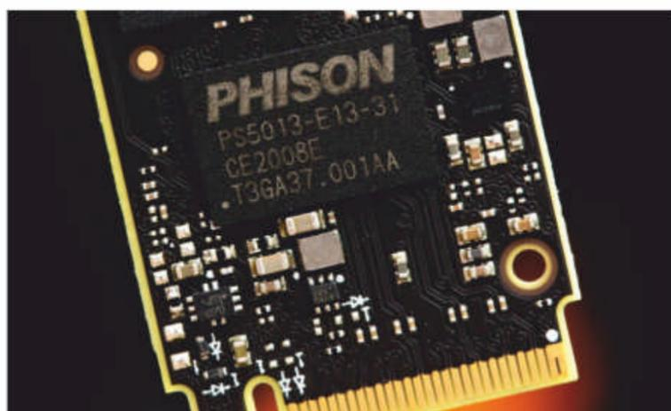
The P2's four TLC 3D NAND flash chips are paired with a third-party Phison PS5013-E13T controller.
