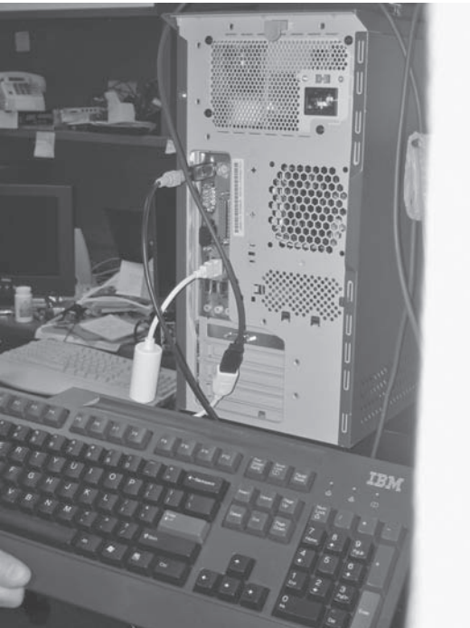
Keyloggers are mechanisms which capture information from installed keylogging devices. Software keyloggers also provide screen-capture features, which users can utilize to view screenshot images of victim activity. Hardware and software keyloggers have varying advantages and disadvantages. Hardware keyloggers can be easily installed and removed. The photo contains two such devices. One is plugged into the USB port and the other connects the keyboard to the CPU. Both devices were generously donated by KeyGhost. (Dr. Marjie T. Britz, Ph.D).
