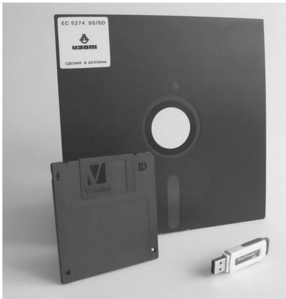
Fig. 12.1 Floppy disks The 8-inch floppy disk was created by IBM's Alan Shugart in 1971. Source: Wikimedia Commons
