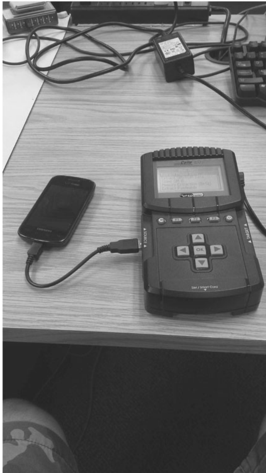
Fig. 14.2 Cellebrite device Cellebrite Universal Forensic Extraction Device (UFED) is a portable device used for forensically extracting data from cell phones. See www.cellebrite.com According to the Cellebrite brochure, the Cellebrite UFED allows for the “complete extraction of existing, hidden, and deleted phone data, including call history, text messages, contacts, images, and geotags.” Source: Photo courtesy of Marcus Thompson, Law Enforcement Coordinator and Instructor for Purdue University’s Cyber Forensics program
