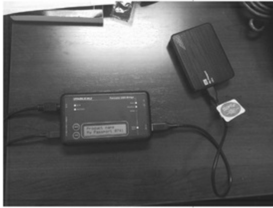
Fig. 13.1a and 13.1b Write blockers A write blocker is a device that allows read-only access to all accessible data on a drive, as well as preventing anything from being written to the original drive, which would alter or modify the original evidence. Figure 13.1a shows an example of a hardware-based write blocker, Tableau T8.
