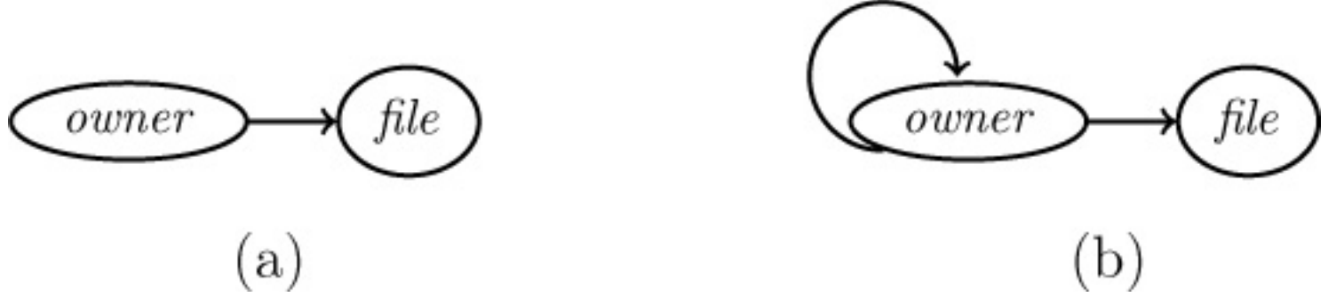
Figure 3–6: Graph (a) corresponds to the cc for the owner-based policy. Graph (b) corresponds to the Take-Grant Protection Model. Both are acyclic; graph (a) is loop-free, but graph (b) contains a loop from one vertex to that same vertex.
