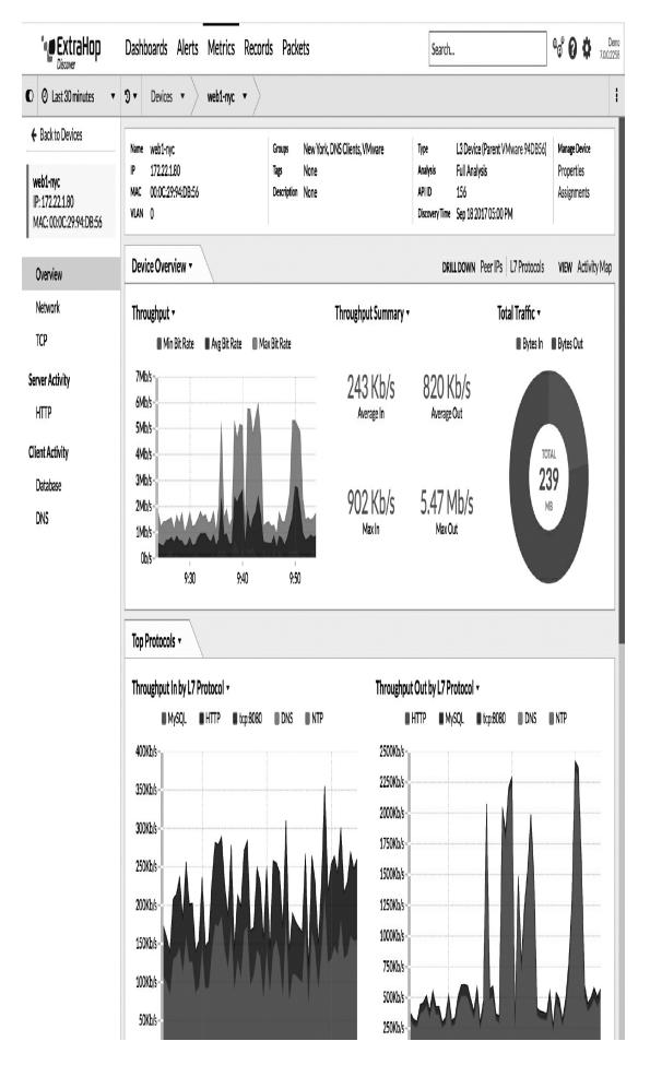
A SIEM tool takes data from the various technical security controls across the organisation, correlates it, and spits the results out onto a (I'm sorry, I'm about to use an overloaded marketing term) single pane of glass display. Essentially, the goal of SIEM is to reduce the number of places the incident responder has to search for information relevant to a potential security incident.
