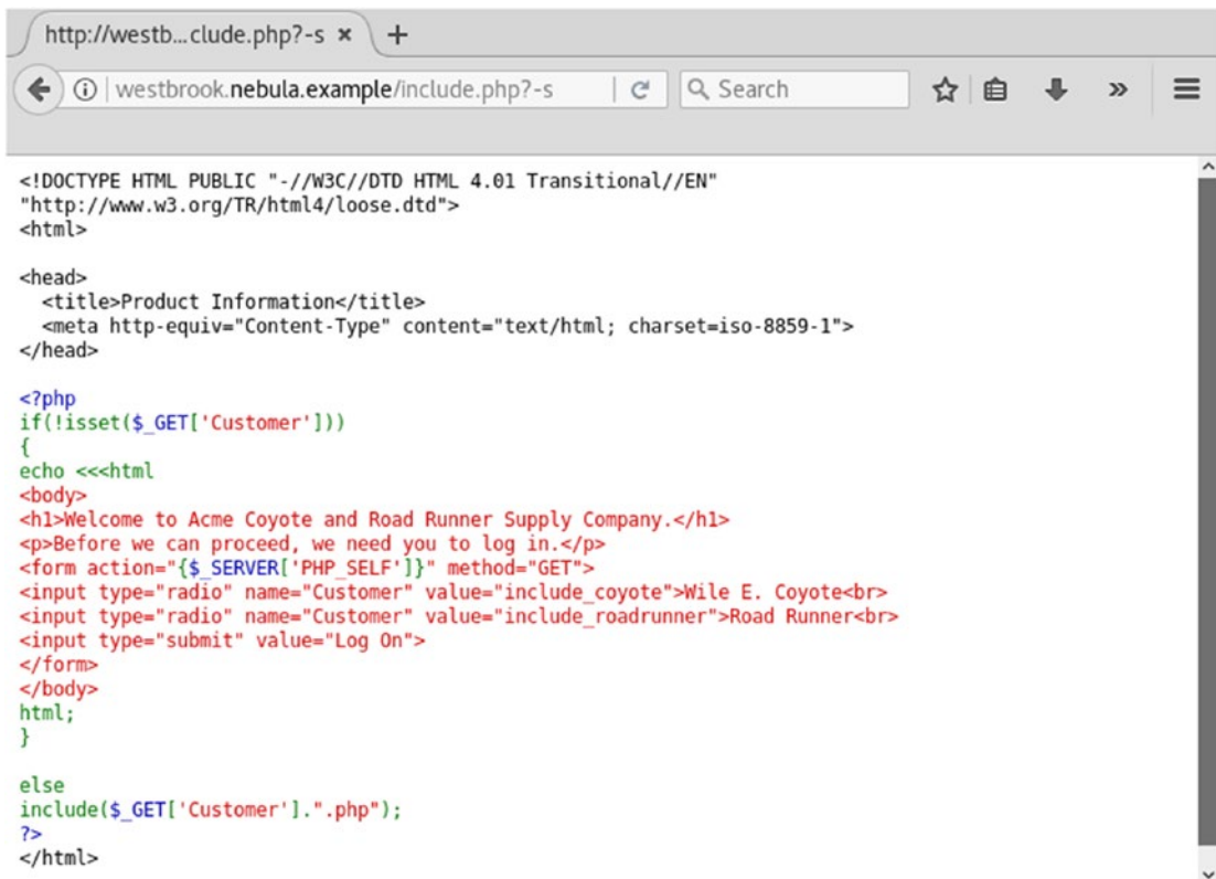
Figure 20-12. Attacking a PHP installation vulnerable to CVE 2012-1823 by requesting a page with the query string “-s”. The target server is Ubuntu 11.04 running PHP as a CGI module. Shown on Kali running Firefox 52.9.
