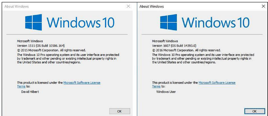
Figure 1-9. The results of the command winver on two different Windows systems. The one on the left is build 1511 and patched through 10586.164; the one on the right is the “Anniversary Update,” build 14393, and is otherwise unpatched.
