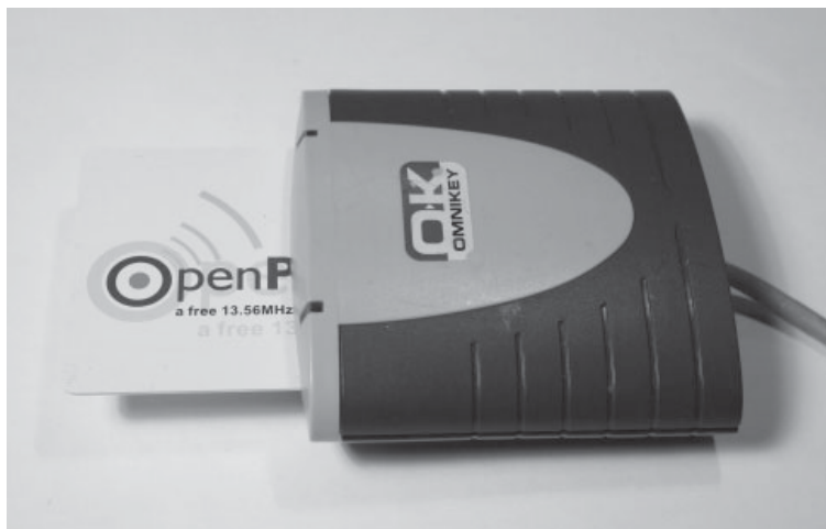
Figure 10-8 OpenPICC smartcard reader
