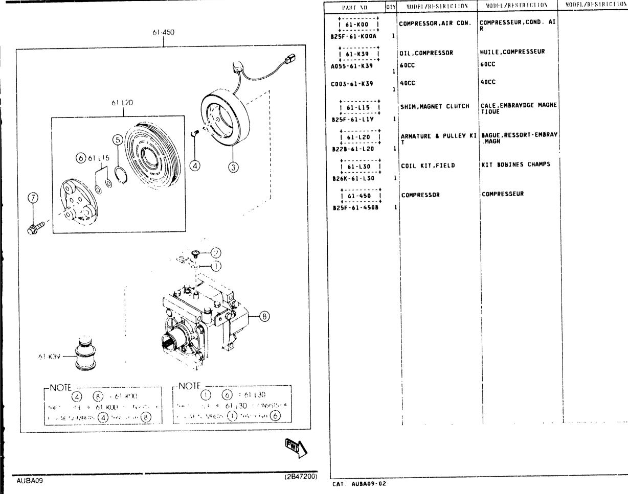
6140B AIR CONDITIONING COMPRESSOR COMPONENTS (2000CC)
