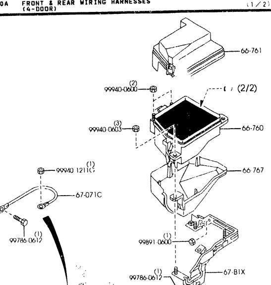
1 18-811A MAIN RELAY CIRCUIT OPENNING RELAY 2 18-821 3 66-136A 40A 4 100A 66-136D (5) 30A 66-497D 6 67-099D 60A ٠,  $\overline{O}$ 7 5A 67-099P 8 10A 67-099P 9 67-099P 15A 4 COMBI LAMP 10 67-7403 RELAY 1 67.7403 HORN RELAY HEAD LAMP (2)67-7403 RELAY AIR CON RELAY (13) 67 7403 COOLING FAN RELAY (1) 67-7403 (WA LOCK BRAKE) 60A (15) 67-099D ADDITIONAL 6 67-7403 FAN RELAY -NOTE (14) > 66-760 (2)THE D-CODE OF 66-760 CONSISTS OF FIGURE NUMBERS (2) THROUGH (14)
