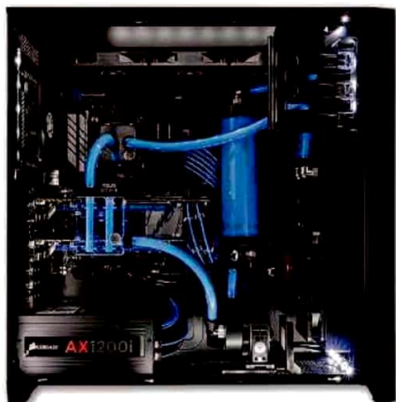
The blue water-cooling tubes help keep this PC Specialist machine quiet
