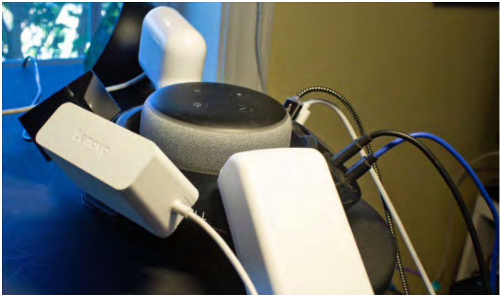
The round form factor and the widely spaced outlets enable the Accell Power Dot to accommodate even oversized AC adapters without blocking adjacent outlets.
