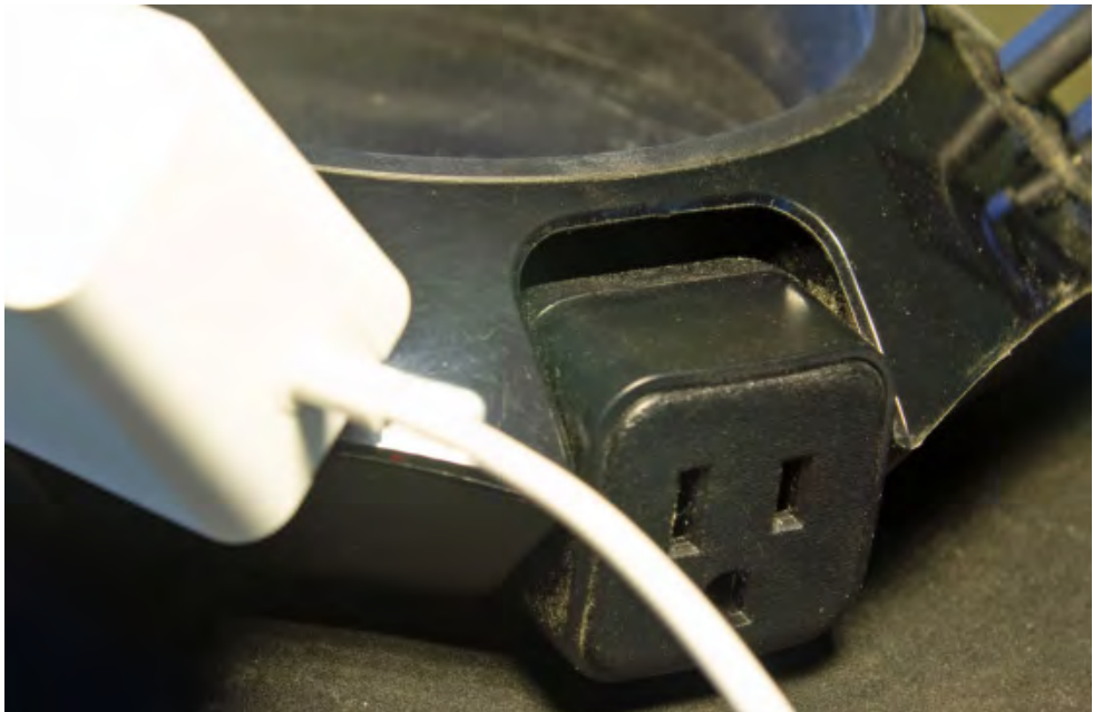
The Power Dot's four outlets pivot, but it takes a lot of force to move them.
