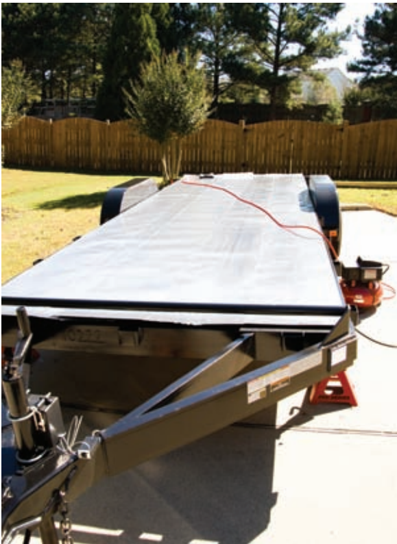
Trailer with Flashing Installed
