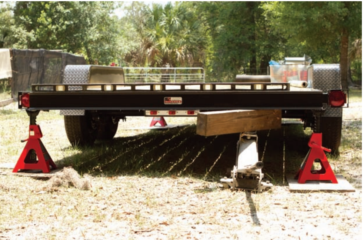
Trailer Being Levelled
