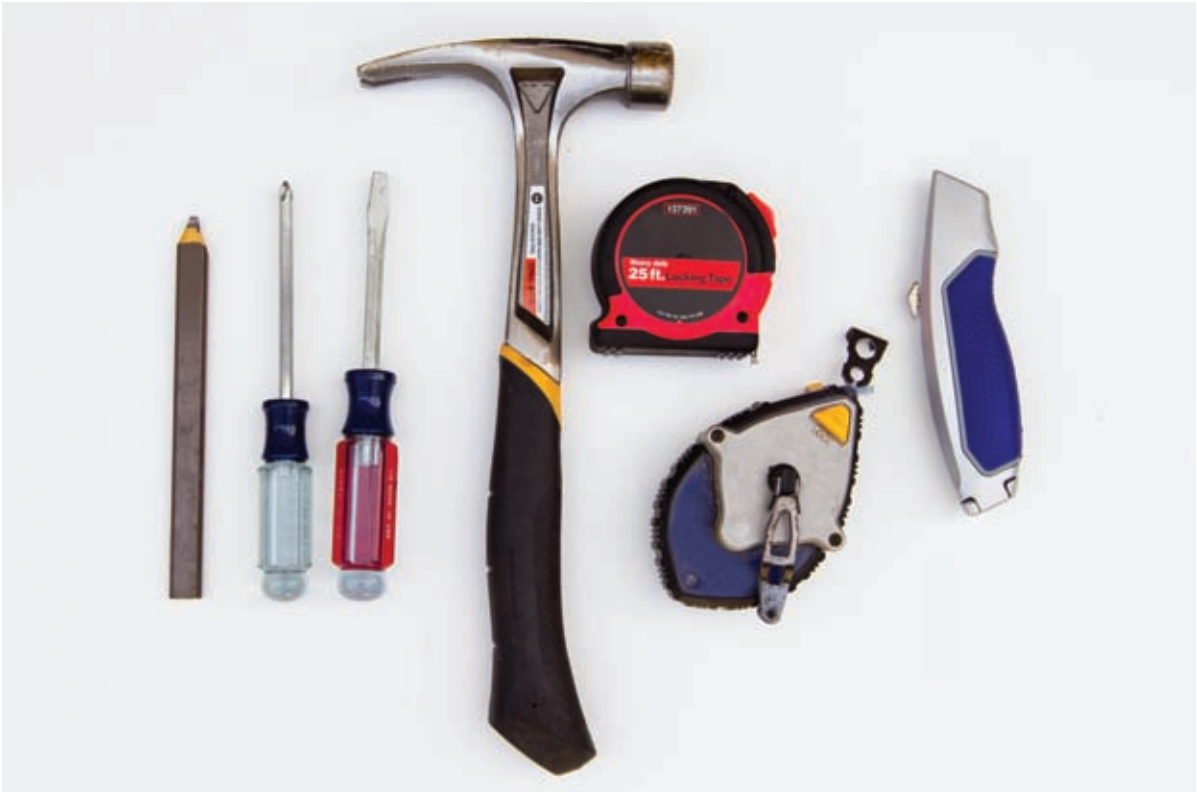
Carpenters Pencil, Screw Drivers, Hammer, Tape Measure, Chalk Line, and Utility Knife
