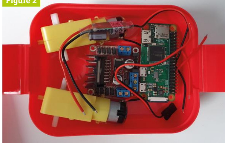
▲ Figure 2 A fundamental step in robot creation is test-fitting where items might go! Use the real components or drawings of them
