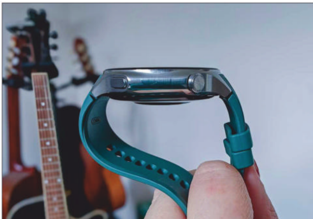
At 12mm thick and a weight of 49g (sans strap), this is a chunky and heavy smartwatch.
