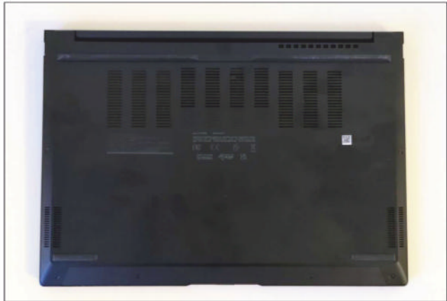
Clear grids for air intakes and speakers on the bottom.
