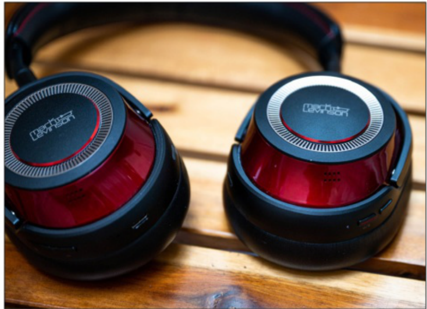
The Mark Levinson No. 5909 is outfitted with microphones inside and outside of each ear cup, four for phone calls and four for active noise cancellation.
