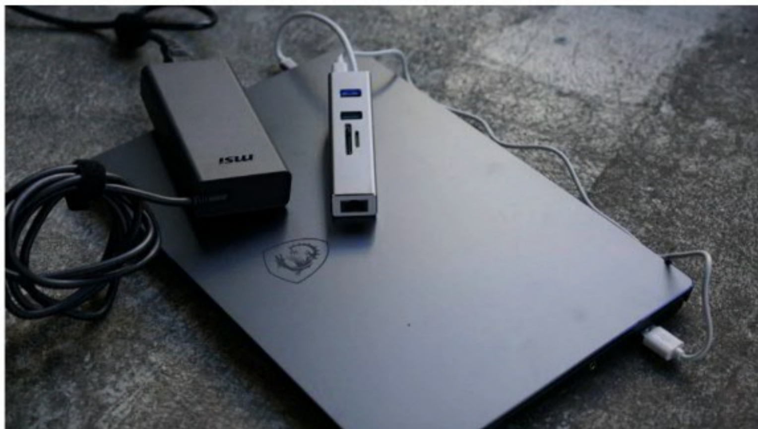
MSI bundles a USB-C dongle with ethernet and USB ports along with a 90 watt USB-C power brick.
