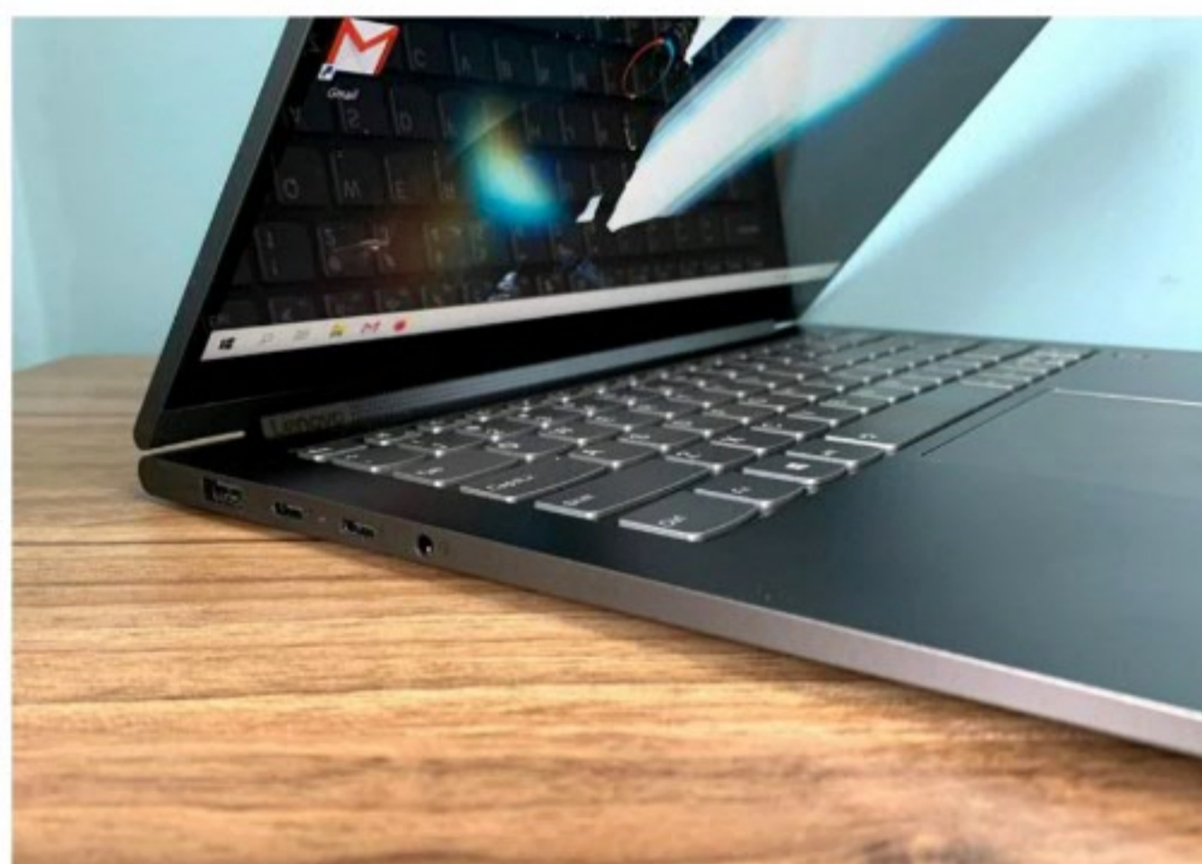
The Lenovo Yoga C940 14 has a USB-A 3.1 port and two USB-C Thunderbolt 3 ports, but they're all on one side.
