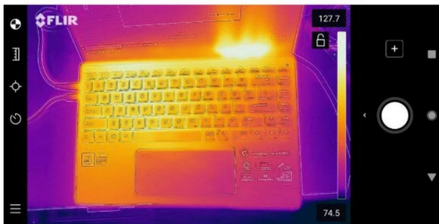
The MSI Prestige 14's single exhaust fan pushes all of the heat out one side of the laptop.
