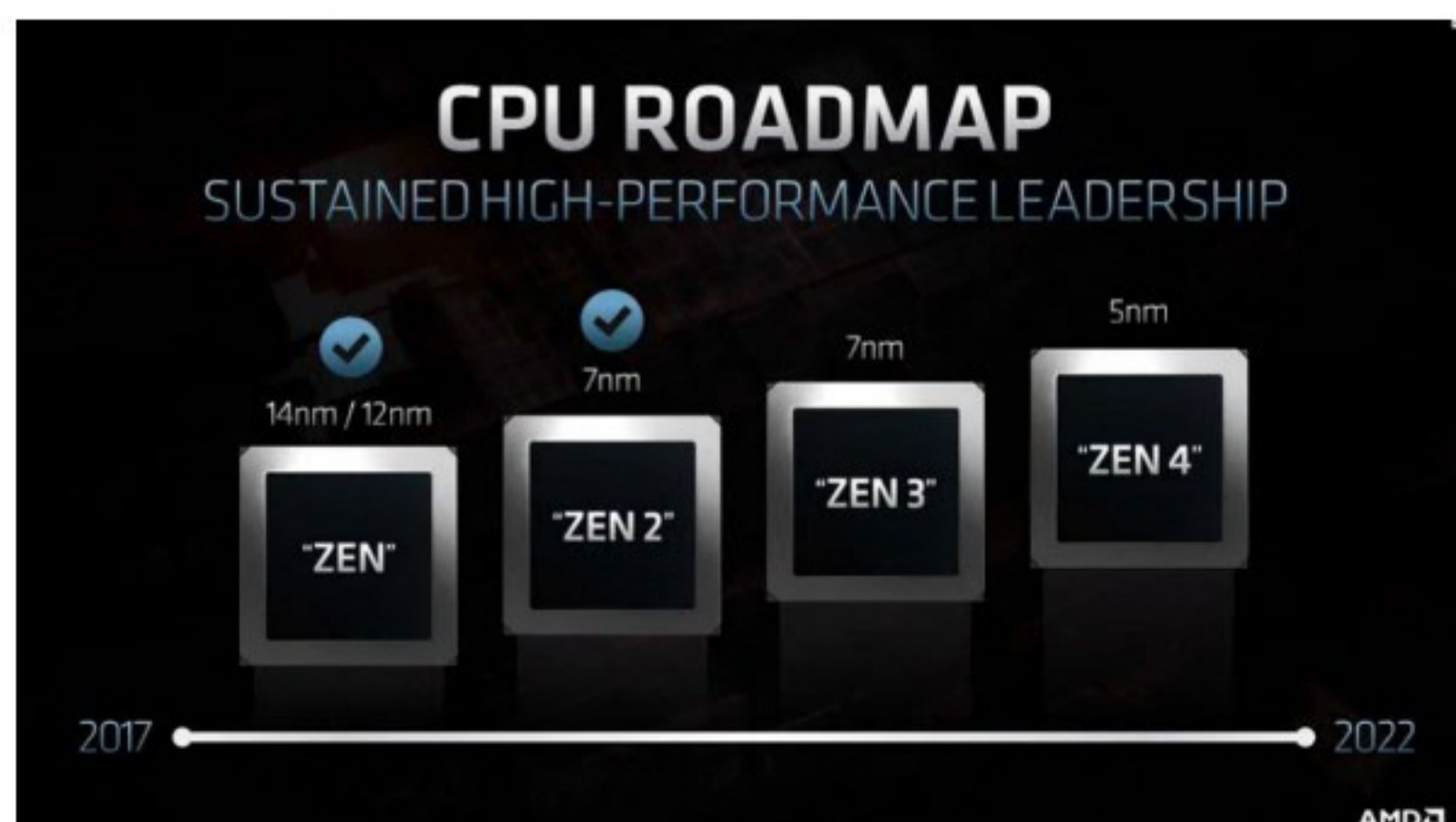
AMD's Zen architecture road map now extends through 2022. Remember, this includes both Epyc products in the datacenter as well as the PC.
