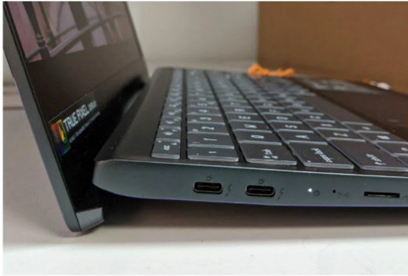
Lifting the lid on the MSI Prestige 14 causes the bottom edge of the panel to tilt the laptop upward, increasing airflow.
