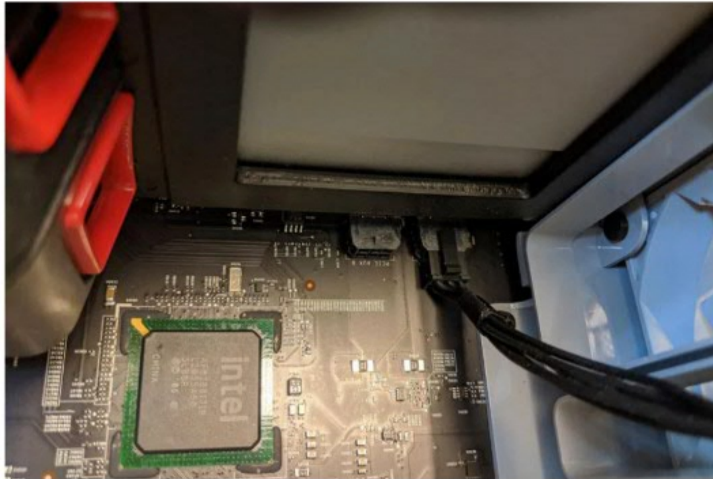
Apple's Mac Pro tower routed power for the GPUs through the motherboard. A similar system will exist in ATX12VO—but only for SATA power connectors.
