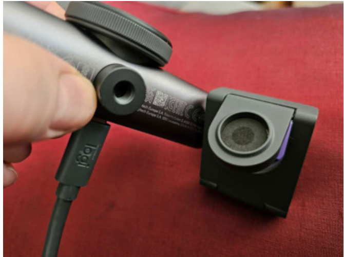
The Logitech MX Brio is connected magnetically to its mount, with a threaded screw hole for an optional third-party stand.
