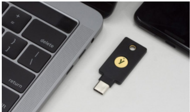
A Fido 2 stick like this is one of several backup options for passkeys. However, the most convenient option is synchronization with the smartphone in the cloud.
