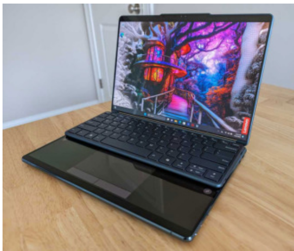
The Bluetooth keyboard magnetically attaches to either the folio stand or the bottom of the laptop itself.
