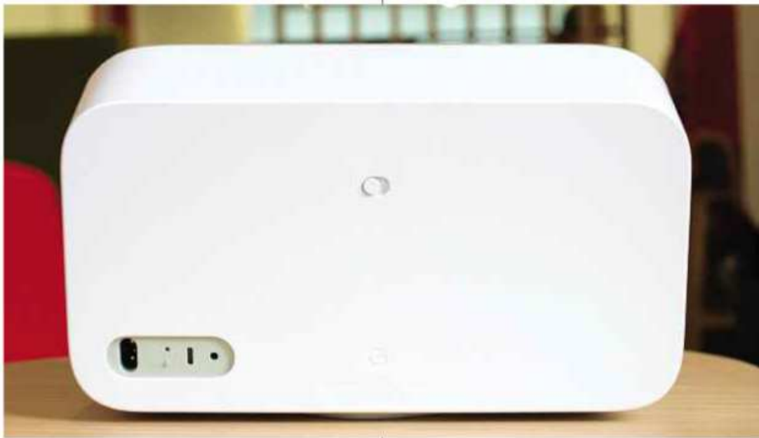
ABOVE At the rear, there’s a USB-C port – but it can’t be used for audio
