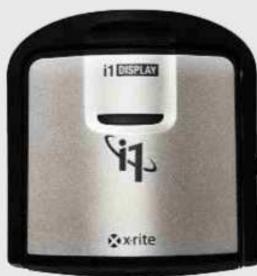
ABOVE We test all screens for brightness and accuracy using an X-Rite i1Display Pro colorimeter
