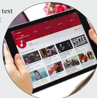
BELOW We play back a video, setting the screen to 170cd/m 2 , until the battery runs out to test battery life
