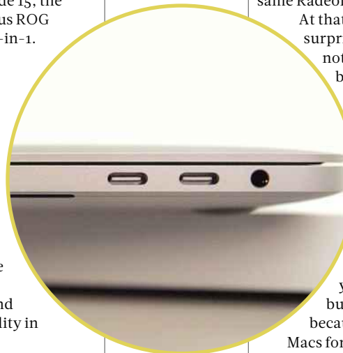
ABOVE The MacBook Pro includes four Thunderbolt 3 ports – two on each side
