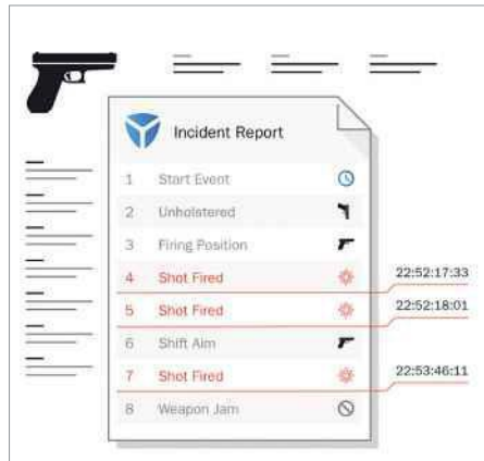
ABOVE Yardarm’s forensic Blackbox system records key details such as when the gun was unholstered, aimed and fired
