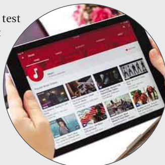
BELOW We play back a video, setting the screen to 170cd/m 2 , until the battery runs out to test battery life
