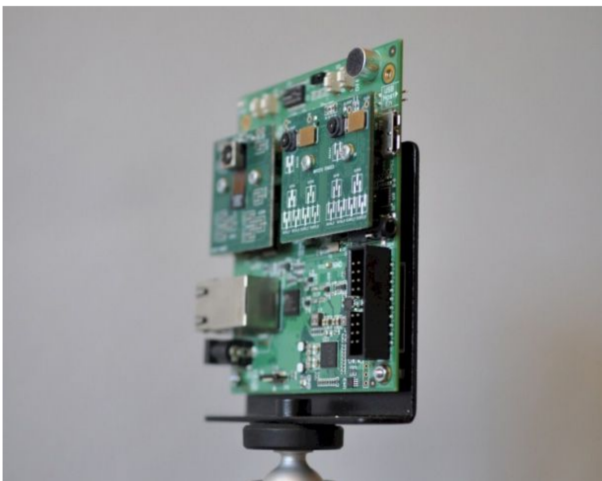
The Movidius Myriad 2 reference board is an always-on vision processor made for power-constrained environments.
