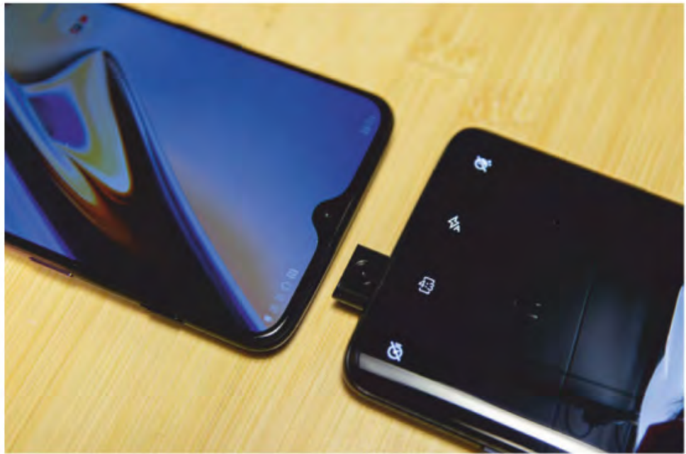
The OnePlus 7 Pro (right) uses a pop-up camera instead of a notch.
