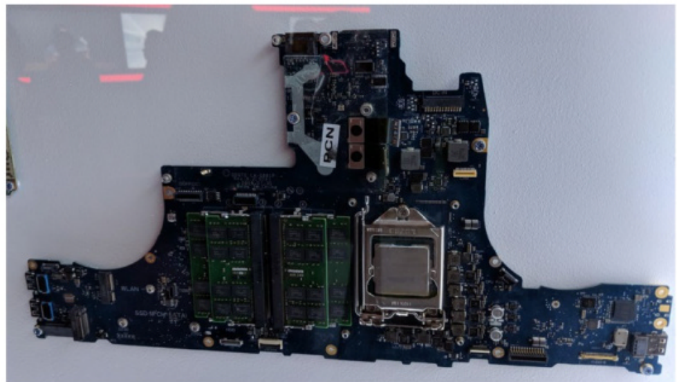
The motherboard of the Alienware Area-51m R1 features four SO-DIMM slots, two M.2 slots, and a standard LGA-1151 socket for the desktop CPU.
