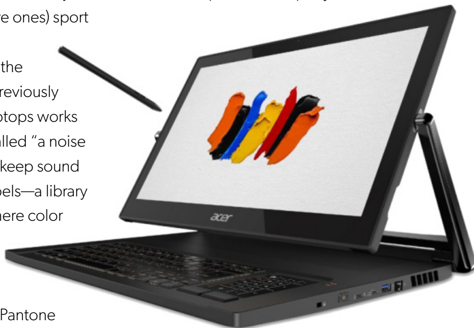
The ConceptD 9 laptop has a display that rotates on a two-armed hinge, and a Wacom EMR pen for its touchscreen.
