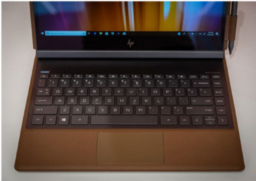
The keyboard has 1.3mm of travel, not bad for a laptop this thin.
