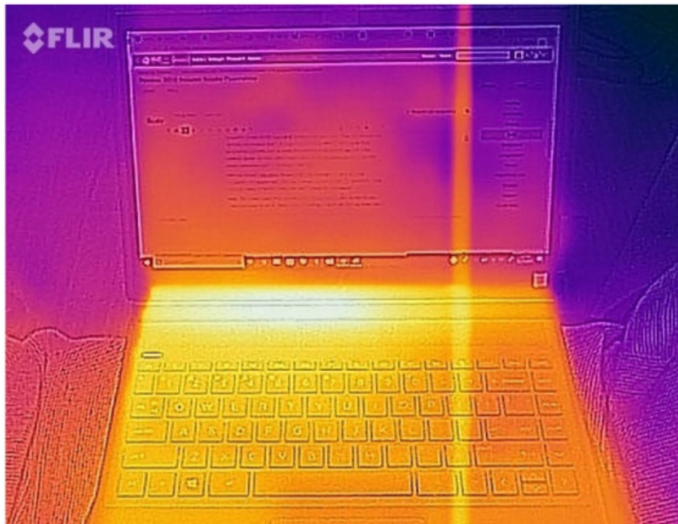
This FLIR heat sensor map shows the hot spot that developed occasionally around the CPU on the HP Spectre Folio's slender motherboard.
