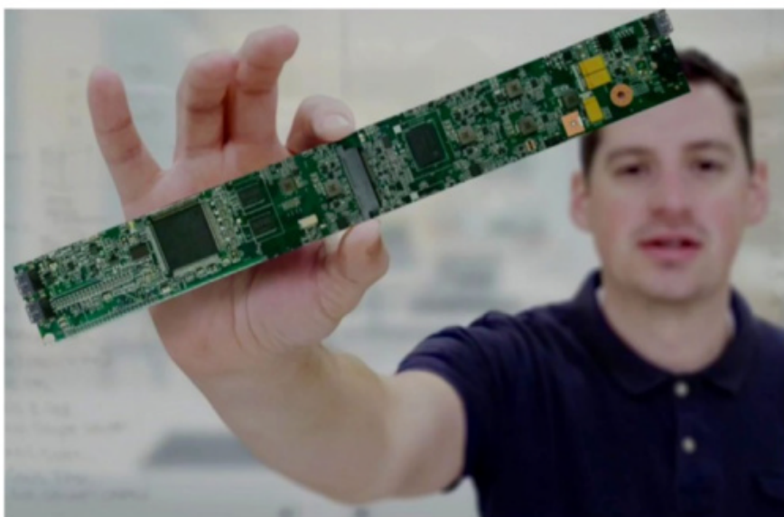
Intel partnered with HP to make the teeny motherboard for the Spectre Folio, a mere strip running along the top of the keyboard.
