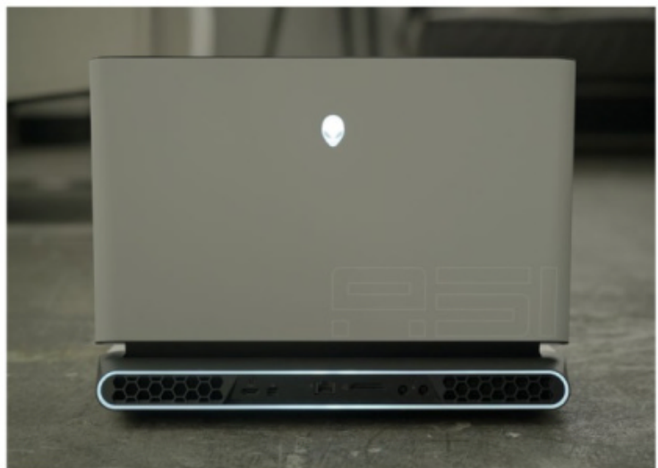
The 2.5Gb Ethernet, Alienware Amplifier, HDMI and miniDisplayPort are routed out the rear of the Area-51m.
