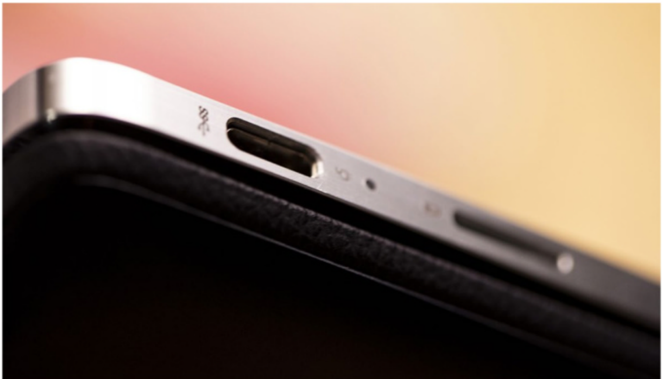
This USB-C port is clearly labeled as a SuperSpeed port which means 5Gbps is its maximum speed.
