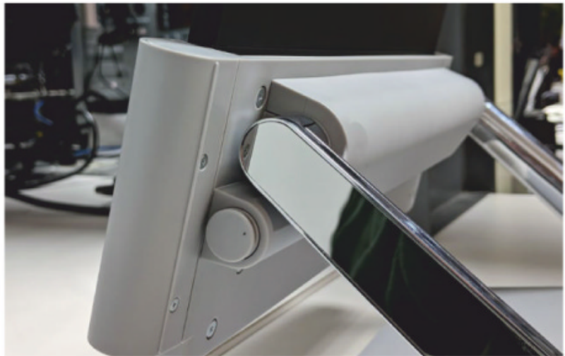
A closer look at the hinges that allow the SD7000 to raise, lower, and swivel the Surface tablet.
