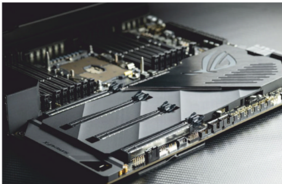
One of two current motherboards for the new 28-core Xeon W-3175X is the Asus Dominus Extreme—a 14x14-inch motherboard using the SSI EEB form factor.
