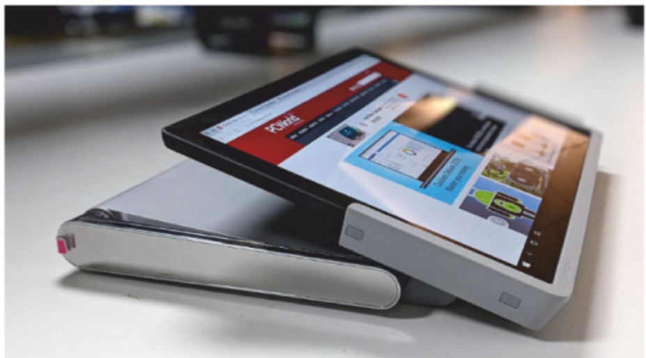
...and here the SD7000 is in “easel mode.” It doesn’t recline as far as the Surface Pro 6 kickstand allows, but it provides a sturdier surface.
