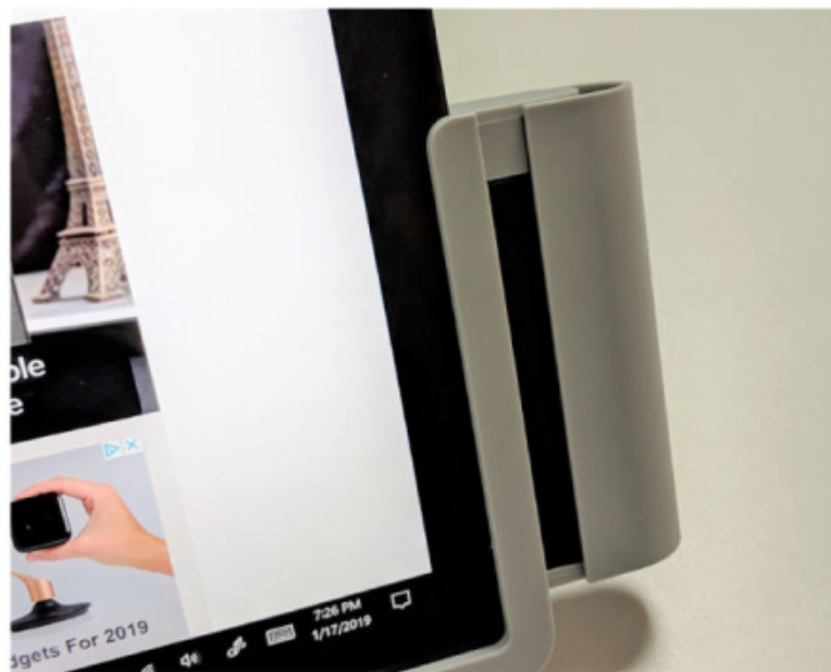
A retaining handle snaps in and out, connecting power and I/O to the Surface tablet and holding it in place.
