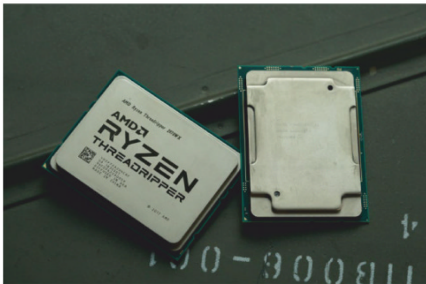
On the right is Intel's new 28-core Xeon W-3175X and on the left for a size comparison is AMD's Threadripper 2970WX.
