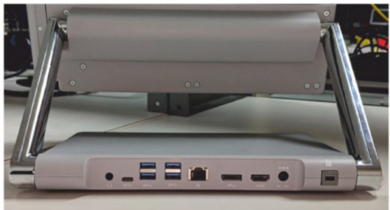
The ports on the rear of the Kensington SD7000. Don't forget the Kensington lock to the far right!
