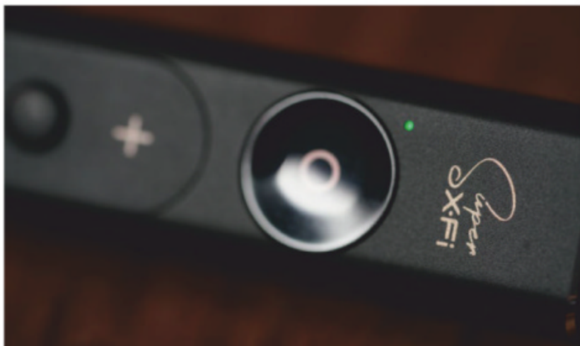
The large round button on the Super X-Fi lets you turn off any processing, making the dongle a standard USB Audio DAC. The LED turns green when processing is on and orange when it's off.
