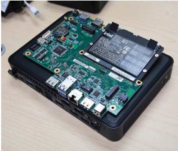
This NUC uses a Compute Element for less compact but more modular design.
