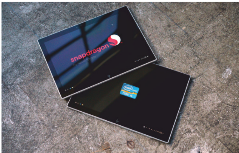
The HP Envy X2 comes in Intel or Qualcomm ARM trim with the only discernible difference being the amount of ports (the Intel version has two USB-C while the Qualcomm one has one USB-C).
