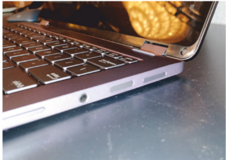
The SIM slot on the side of the 8cx reference notebook.
