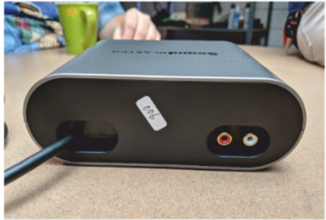
The rear of the new AE-9 breakout box likely features two RCA analog ports.
