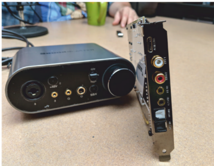
The card appears to have standard 3.5mm jacks for rear, center, and sub, as well as RCA stereo-out and optical-in and -out ports.
