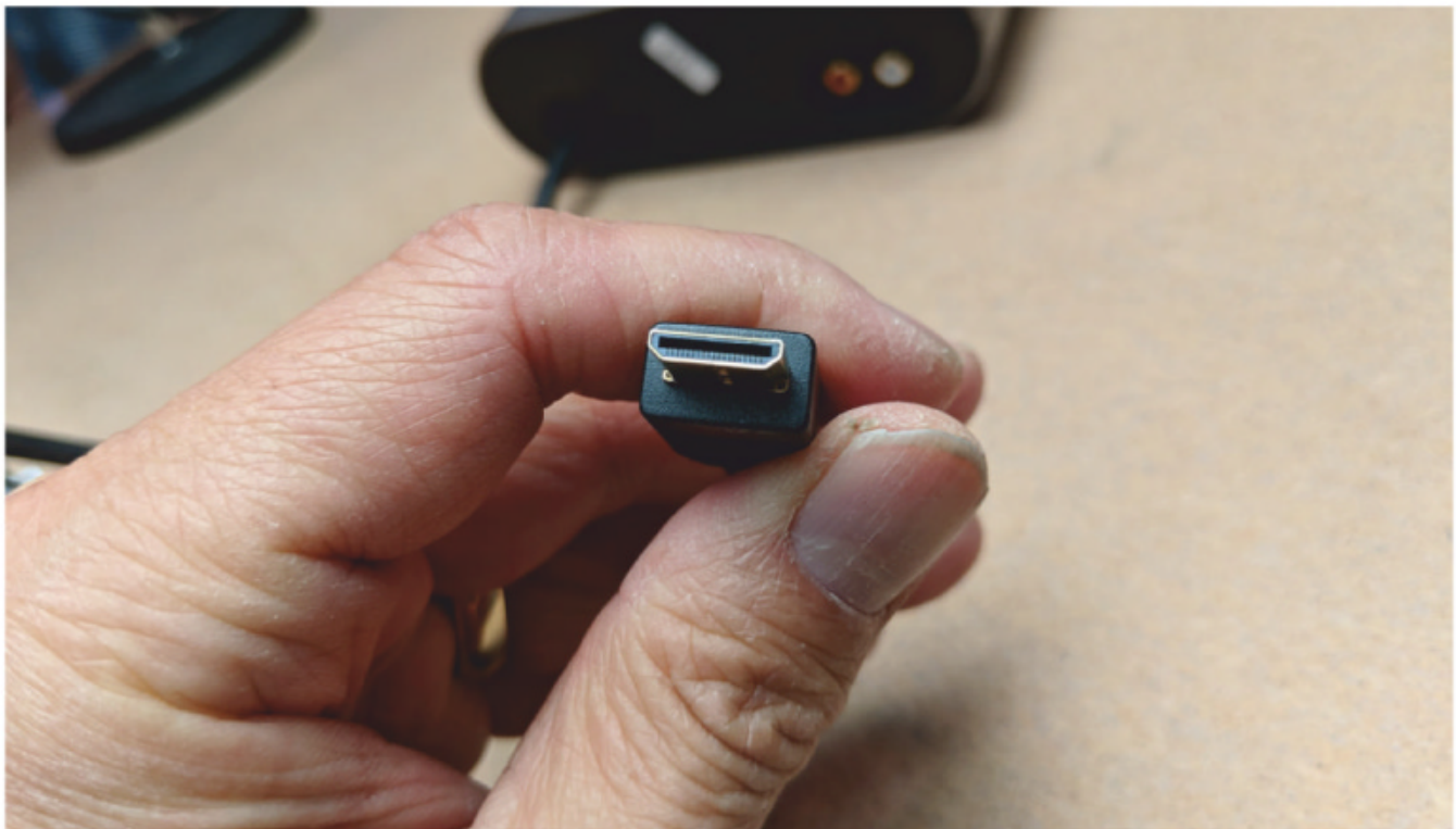
A single cable that connects the Sound Blaster AE-9 to the breakout box looks awfully similar to a mini-HDMI connector.
