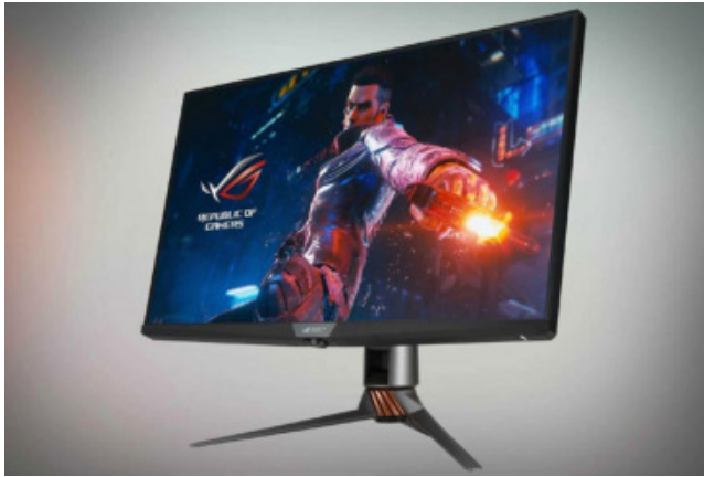
Asus's awesome ROG Swift PG32UQX uses Mini-LED technology and has a massive 1,152 lighting zones.
