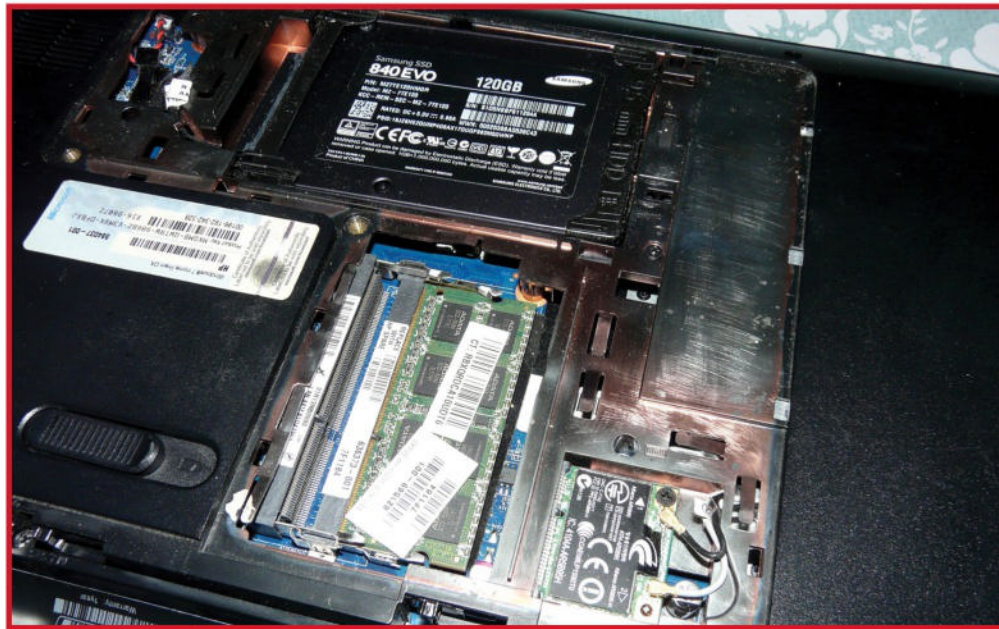
Extra RAM and an SSD drive can do wonders for an aging laptop.
