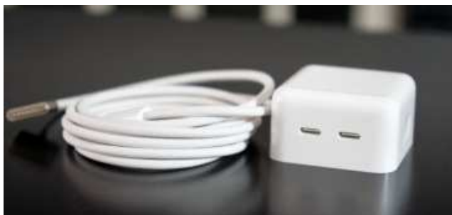
The M2 MacBook Air comes with a nice braided MagSafe cable and compact 35W dual-USB-C Power Adapter (in all but the base configuration).
