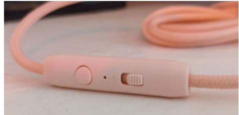
The round button is multifunction, while the pinhole is the microphone.
