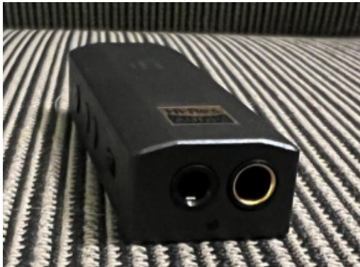
The iFi Go Bar includes jacks for 3.5mm or 4.4mm headphone connectors.
