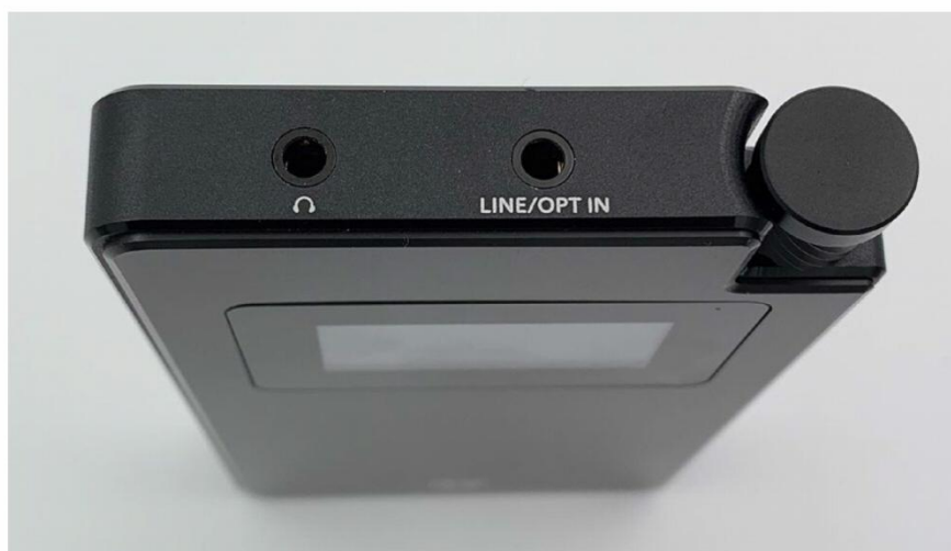
Detail view of the Monolith's top with 3.5mm input and headphone output.
