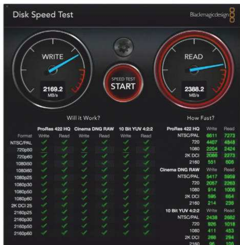
Black Magic's Disk Speed measures only large file transfers. Note: NVMe over Thunderbolt is only slightly slower than internal NVMe. Larger numbers are better.
