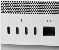
The Mac Studio is festooned with ports, including four Thunderbolt 4 ports on the rear as well as 10Gb Ethernet.
