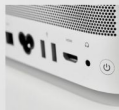
You also get two USB-A ports and an HDMI port, as well as a 3.5mm headphone jack.
