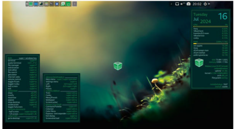
Mabox makes good use of Conky to display useful keyboard shortcuts and key system stats such as RAM and CPU usage.
