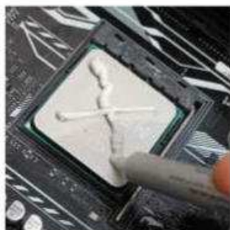
Reapplying your TIM can make a huge difference to CPU temperatures
